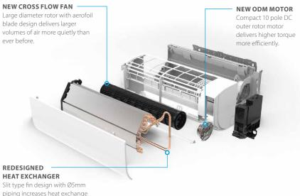
Slit type fin design with Ø5mm piping increases heat exchange area for improved capacity output and energy performance.
